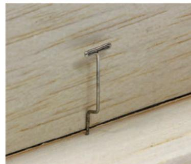
If you need to pin something to your building board but the head of the pin prevents it from fitting tightly against an adjacent surface, try this. With Z-bend pliers, bend your pin to offset the head. With the pin bent this way, it can be inserted through the wood and straight down into the building board, even if it has to sit flush against a vertical section.
